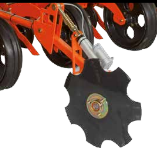
The optional pre-emergence markers assist first spraying operations before seed emergence
