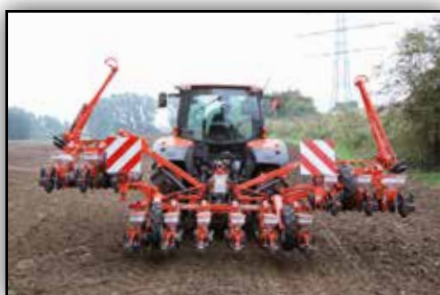
MP1600F - Folding sequence from transport width (<3m) to working width 6m
