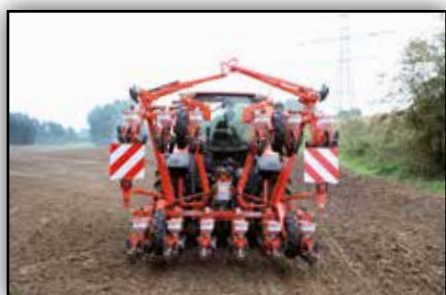
MP1600F - Folding sequence from transport width (<3m) to working width 6m
